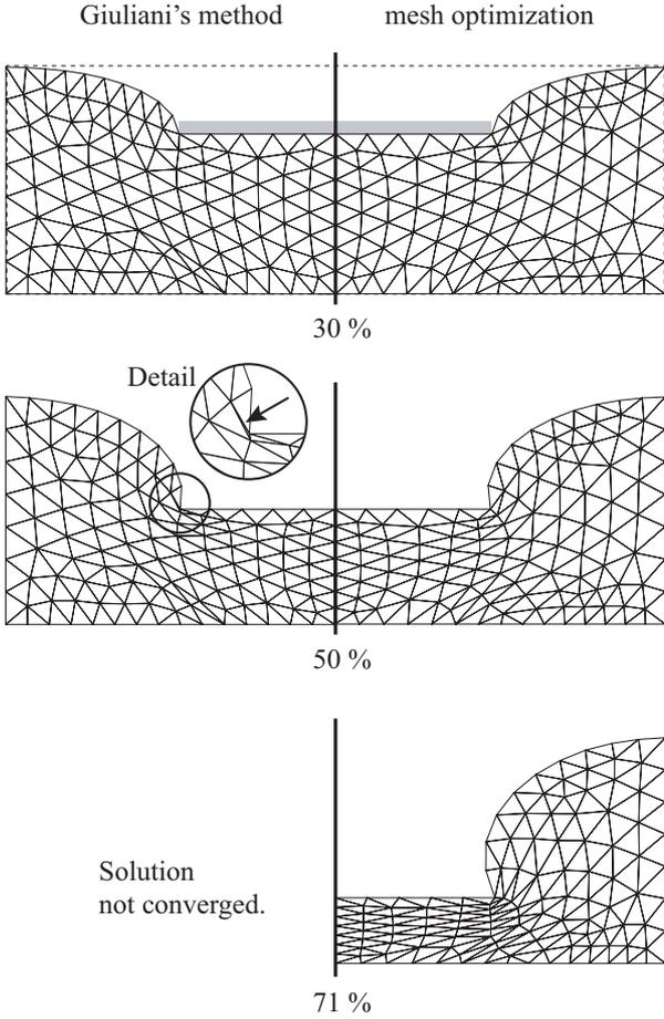
Figure 1: Comparison of Giuliani’s method (*left*) and the current mesh optimization scheme (*right*) applied to back extrusion at different indentations.
