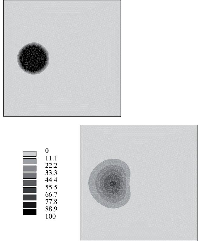
Figure 2: Molenkamp test of the advection algorithm. Initial distribution of the color function (*above*), distribution after a full clockwise rotation (720 steps) of the material about the domain center (*below*).
