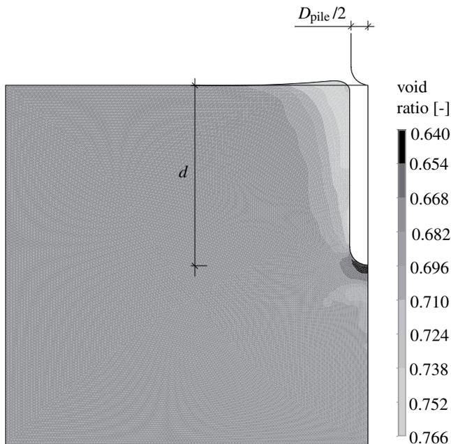
Figure 3: Penetration of a smooth rigid pile into sand (initial void ratio  $e_0 = 0.678$  ( $D_r = 0.34$ )). Edges of the undeformed configuration, and void ratio distribution at a relative penetration depth of  $d/D_{\text{pile}} = 5.0$ .
