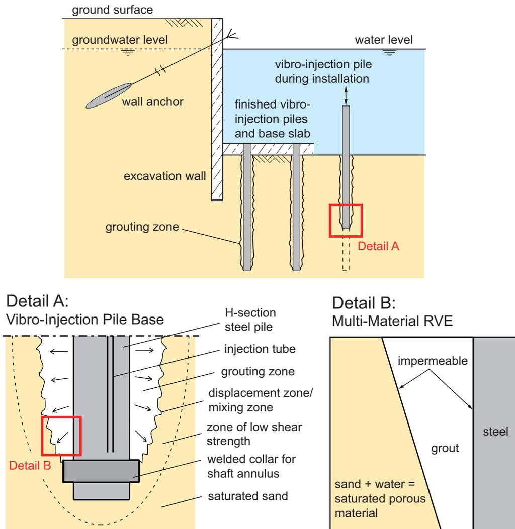
Figure 1: Vibro-Injection Pile Installation in Saturated Sand for a Typical Deep Excavation in Urban Area. Detail A: Phenomenology at the Pile Base. Detail B: Representative Volume Element (RVE).
