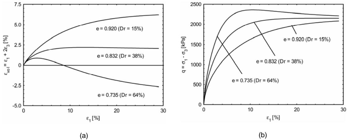
Figure 2. Dilative behaviour of sand under drained triaxial compression: dependency on the density state. Toyoura sand,  $p'_0 = 1000$  kPa.
