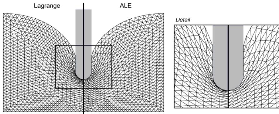
Figure 5. Numerical simulation of the penetration of a smooth rigid pile into elastic material. left: Lagrangian mesh, right: ALE mesh with energy-based regularisation.
