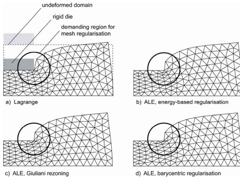
Figure 3. Comparison of different mesh smoothing schemes applied to the numerical simulation of a coining test at the stage of 50 % indentation. (a) Lagrangian mesh and ALE mesh with (b) energy-based regularisation, (c) Giuliani rezoning, (d) barycentric regularisation.
