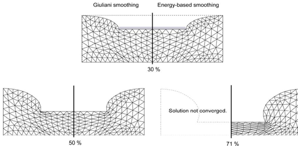
Figure 4. Comparison of Giuliani rezoning and energy-based regularisation applied to the numerical simulation of a back extrusion problem at different indentations.
